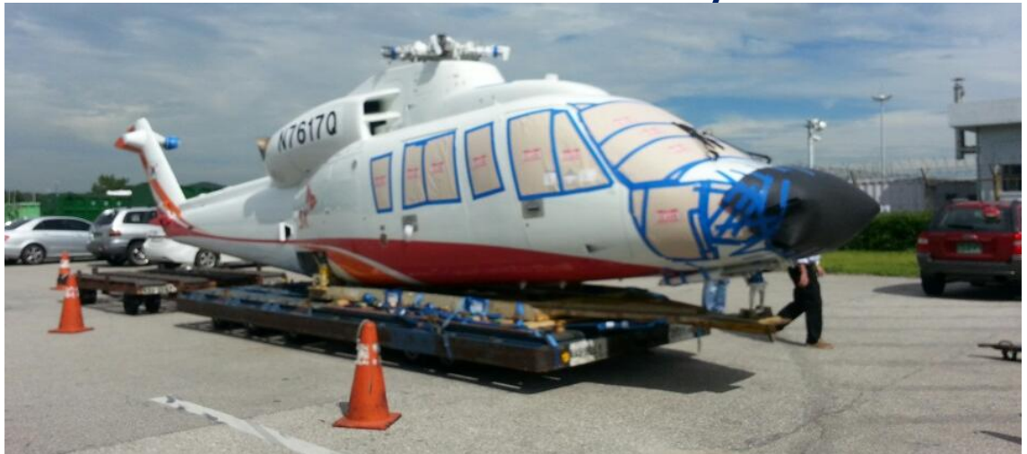
Above: The Sikorsky S-76 D, Size of main fuselage 508"x84"x118" Weight 3,307 kg
